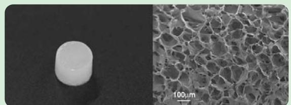
Fig. 3: A porous 3D structure is formed by the addition of a small amount of aqueous organic solvent to silk fibroin solution, followed by freezing and melting processes. (photograph provided by Dr. Yasushi Tamada at NIAS)
