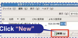
Fig. 2: Virtual Machine Manager Clicking the "New" button initiates the wizard for installing the guest OS, as shown in Fig. 3.
